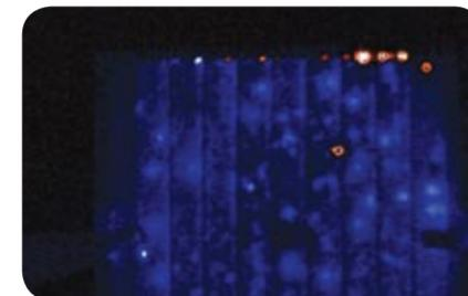
Figure 9. Image of the same solar cell in Figure 2, now showing shunt defects more clearly (orange areas) when mapped with an LIT technique, using the MoviTHERM’s “SolarCheck” system.
