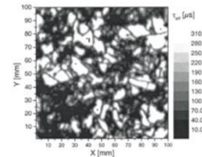
Figure 14. Spatial map of PV cell area showing effective carrier lifetimes ( $\tau_{eff}$ ) in microseconds.
