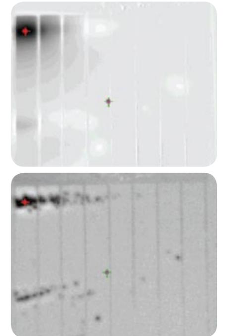
Figure 11. LIT phase images intended to show shunt defects. Note that in the top view (10Hz stimulation) many defects are all but invisible. They show up clearly in the bottom view as dark areas with 200Hz stimulation.
