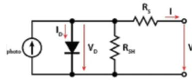
Figure 1. Circuit model of a PV cell.
