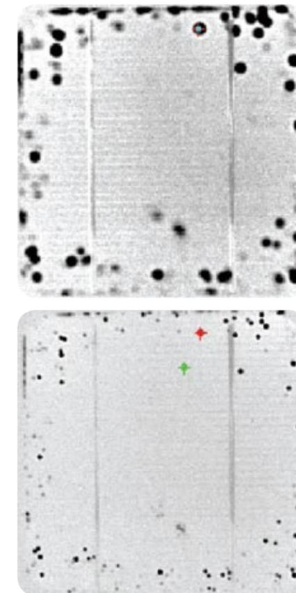
Figure 10. Phase images of shunt defects from lock-in measurements performed with the SolarCheck system at 10Hz (top) and 200Hz (bottom) sine wave stimulation.
