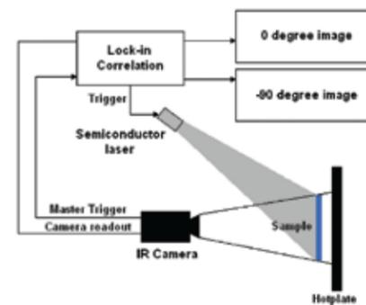
Figure 13. Block diagram of a Carrier Density Imaging system using LIT based on the SolarCheck system.
