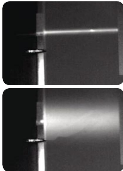
Figure 5. Top: a solar panel being exposed to a short laser pulse, shown as a bright white horizontal line at  $t = 0\text{ms}$  on the crystalline PV cell. Bottom: the same PV cell at  $t = 200\text{ms}$  after laser exposure and heat propagation. The lighter area with the irregular boundary line clearly reveals a crack.
