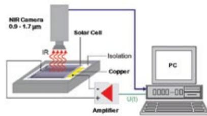
Figure 6. Measurement setup for “Emission Analysis” using MoviTHERM’s IR-NDT system “SolarCheck”. The PV cell (or solar panel) is being electrically stimulated (electroluminescence technique).
