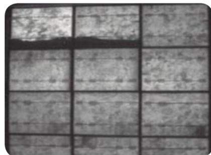
Figure 7. Image of solar cell defects identified through “Emission Analysis”. This image results from the test setup in Figure 6. The dark areas near the bottom of two cells in the upper left represent defects.
