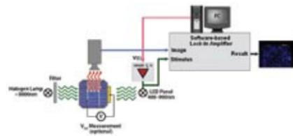
Figure 12. Non-contact LIT test configuration using modulated light as the PV cell stimulus. Optional  $V_{OC}$  measurements do require electrical probing of the cell.
